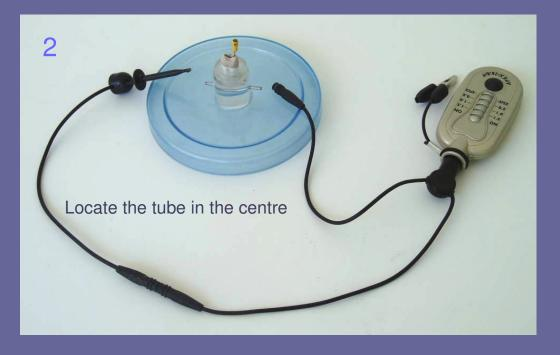
Connect the lip hook socket to the stainless steel pin on the test tube, and connect the file holder to the file (NiTi or regular)
